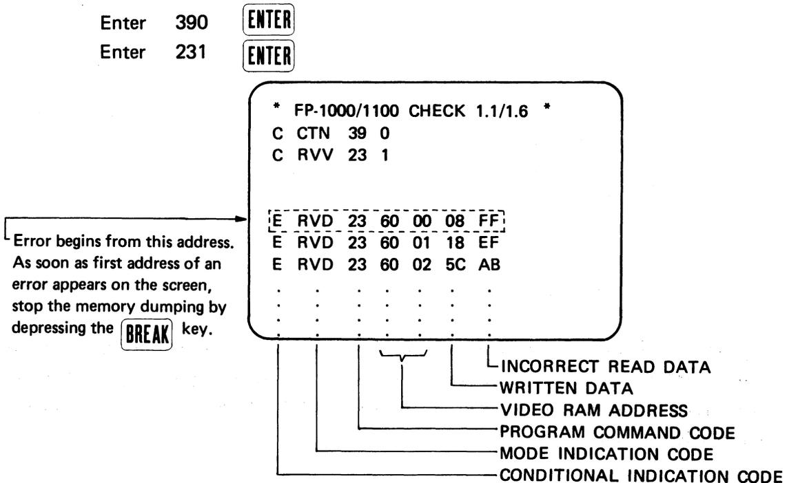
Fig. 10-11 ERROR DISPLAY MODE
