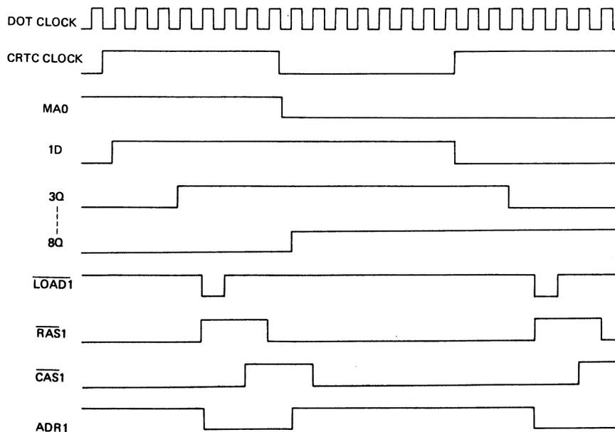
Fig. 8-11 TIMING GENERATE CIRCUIT (I)
