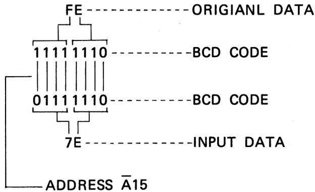
As shown above, the input bit which differs from the original bit is the 1st bit from the left in this case, that is, address  $\bar{A}15$  is the cause of the error.
