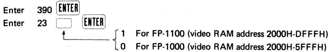
This display mode shows no error in the video RAM memory circuit.
