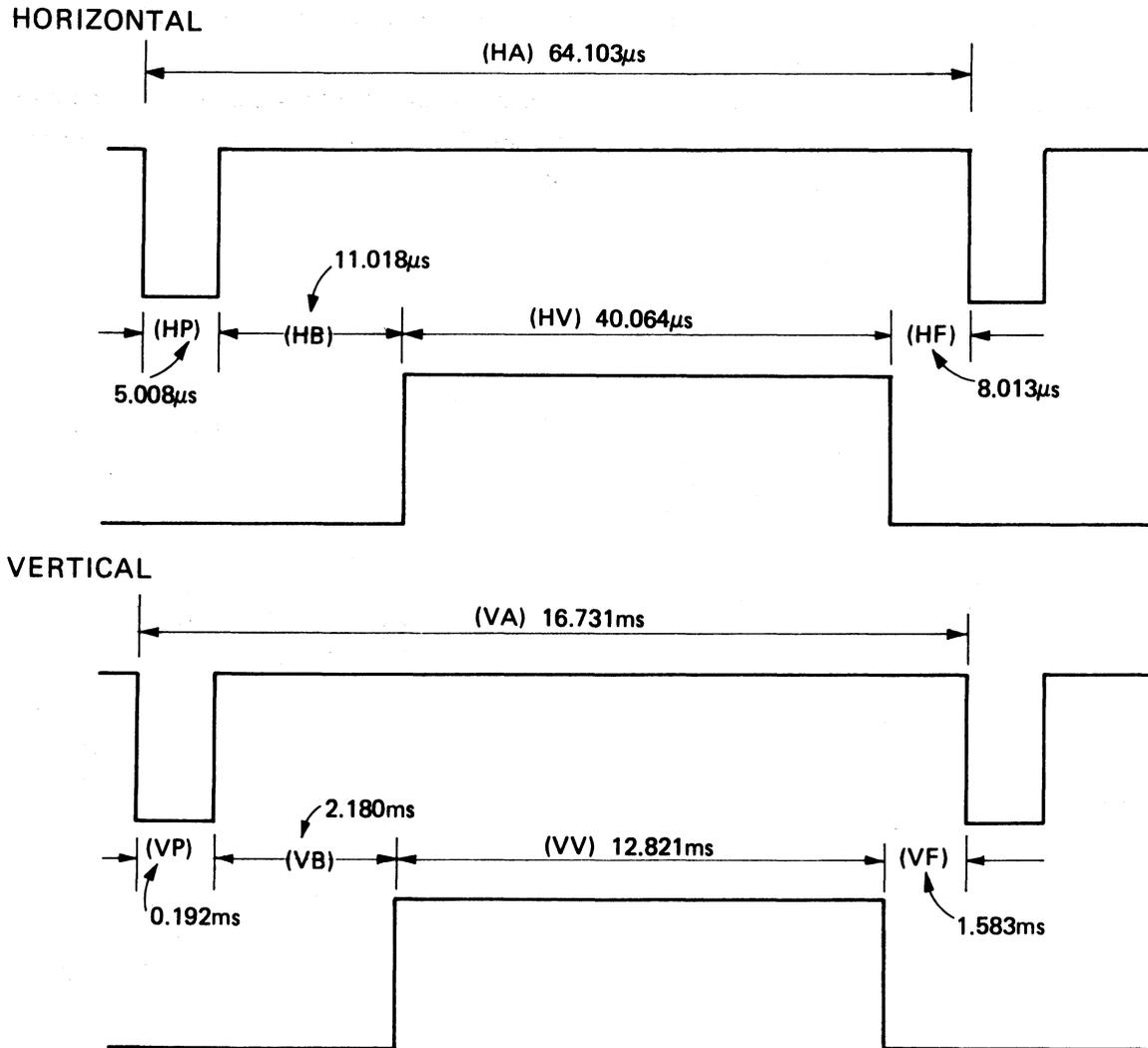
**Fig. 8-13 DISPLAY SYNCHRONIZING SIGNAL**
