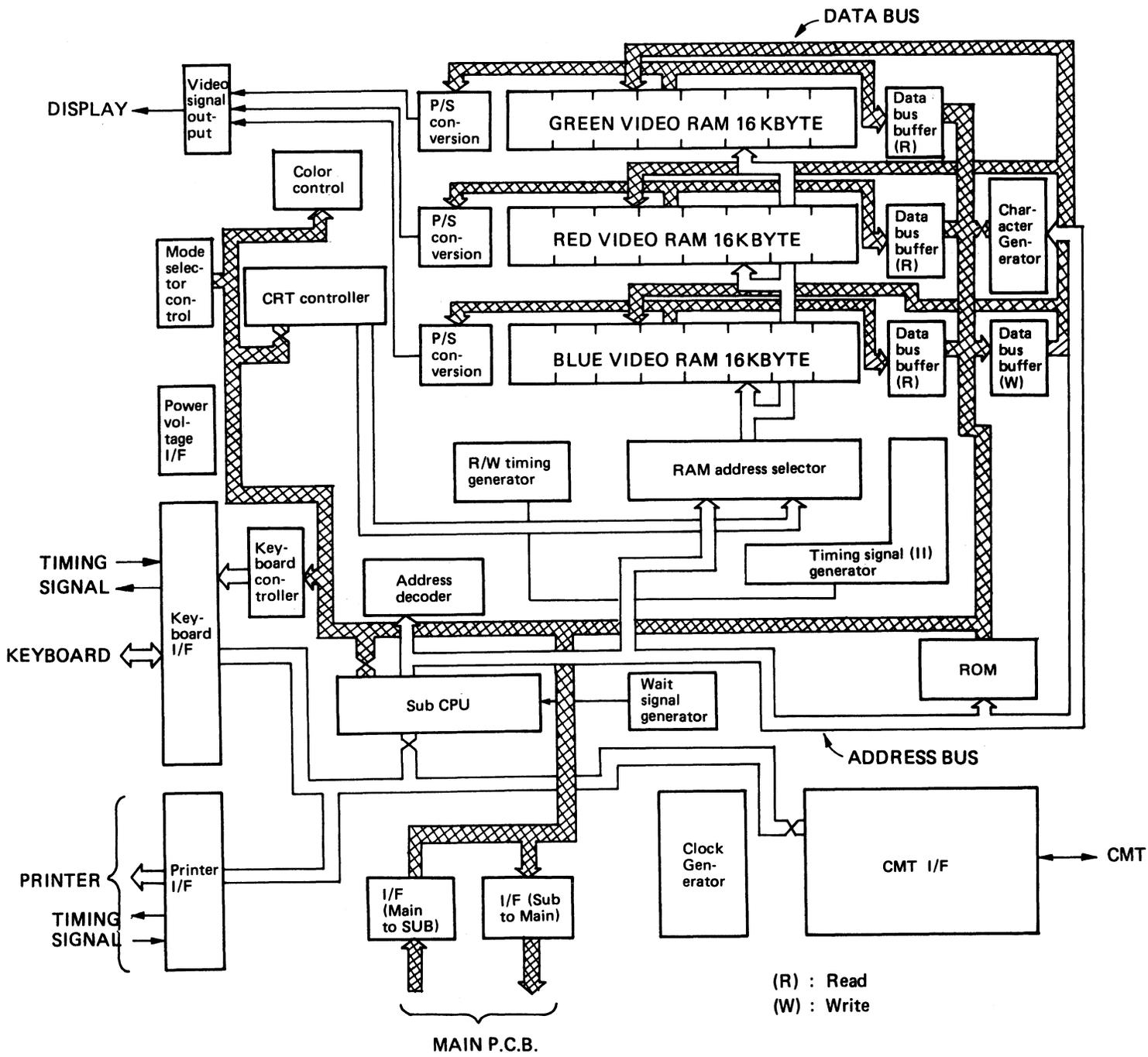
Fig. 2-2 SUB P.C.B. BLOCK DIAGRAM
