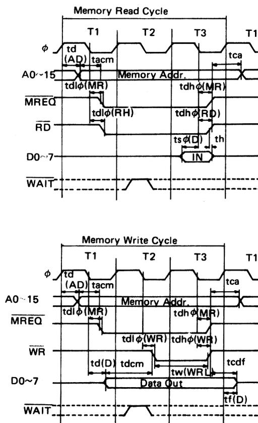
**Fig. 5-2 MEMORY READ/WRITE CYCLE**
