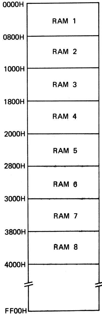
NOTE: RAM 1, RAM 2 . . . RAM 8 in the above memory map designate each RAM chip on the circuit board of the C16K RAM memory pack.
