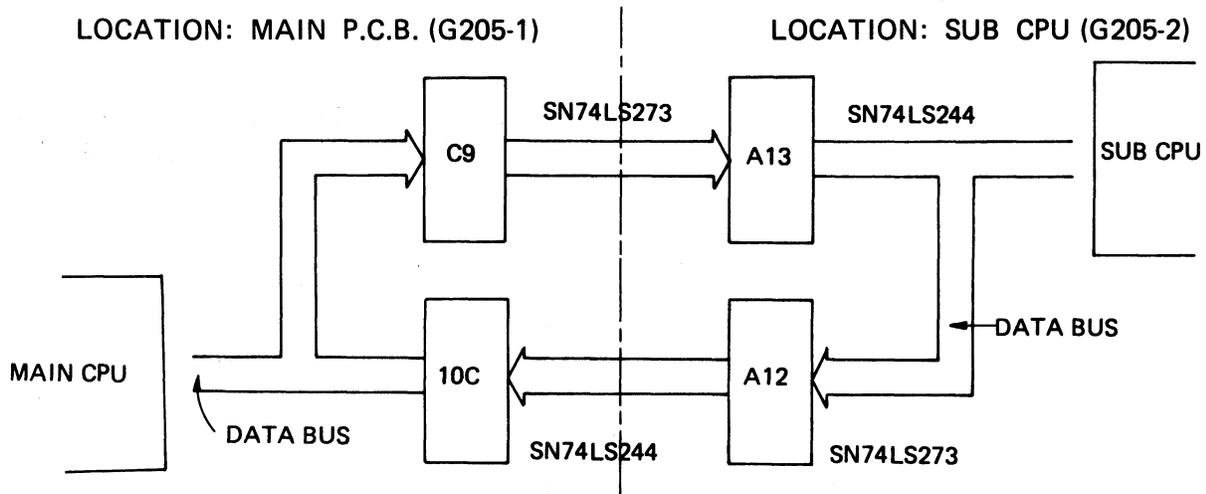
Address for read and write of the data by the main CPU to the latches are as follows.
