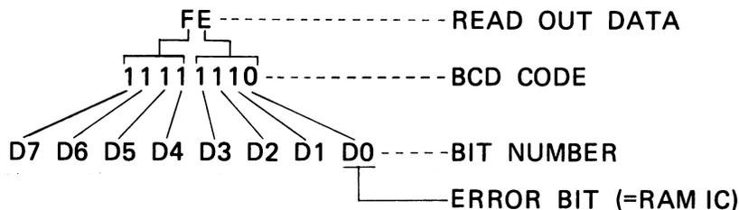
Suppose all RAMs and its circuit are normal, read out data will be "11111111" which is the reversed data of "00000000".
