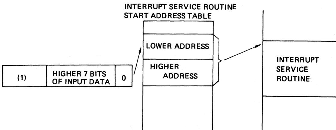
First, start address table for interrupt service routine is accessed by 16 bits which consists of higher 8 bits of the I register content and lower 8 bits of read data (normally the lowest bit is 0). Second, it jumps over to interrupt service routine based on the contents of the selected start address table.
