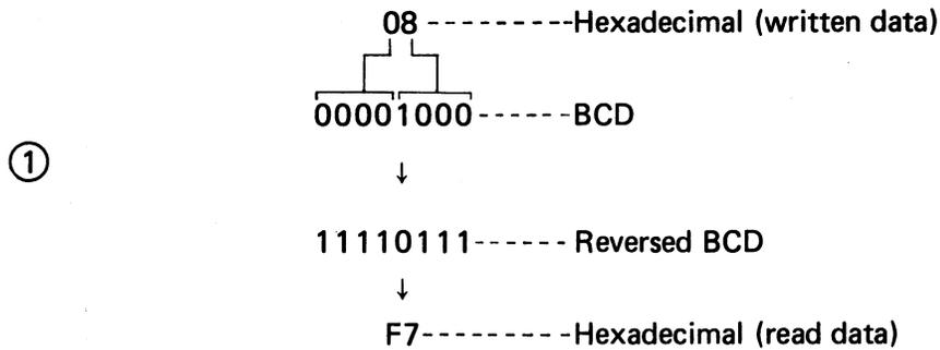
As shown, if the RAM IC is normal, reversed data (bit) of written data "08" should be "F7" instead "FF" and indicated next to the written data on the screen.
