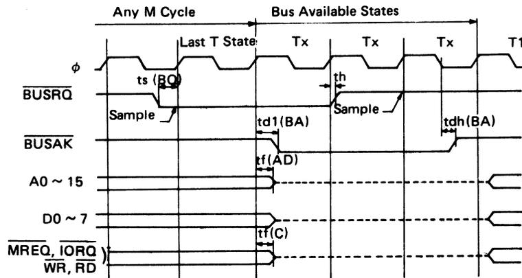
**Fig. 5-4 BUS REQUEST/ACKNOWLEDGE CYCLE**
