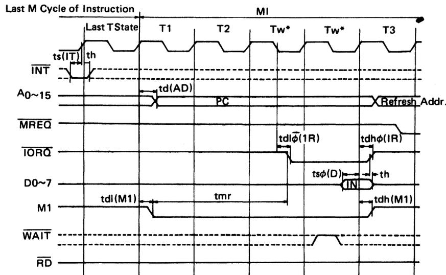
Fig. 5-6 INTERRUPT REQUEST/ACKNOWLEDGE-CYCLE
