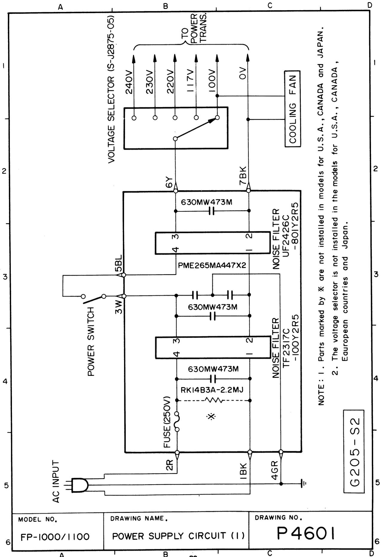
NOTE: 1. Parts marked with \* are not installed in models for U.S.A., CANADA and JAPAN.
