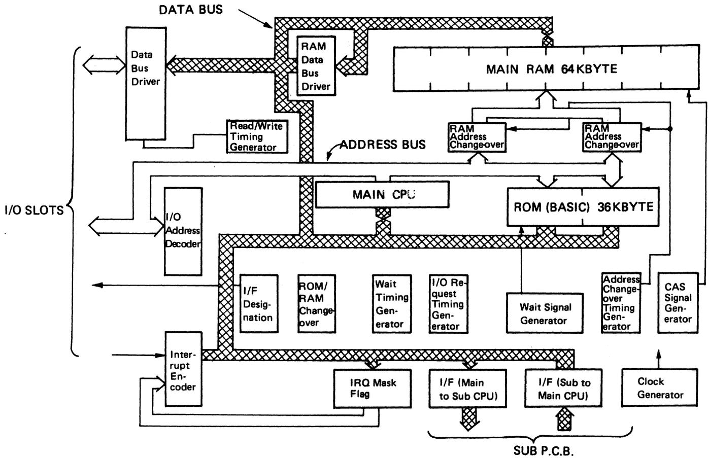
Fig. 2-1 MAIN P.C.B. BLOCK DIAGRAM
