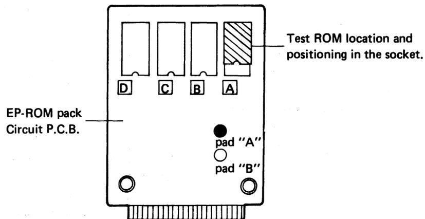
Fig. 10-1 EP-ROM PACK CIRCUIT BOARD
