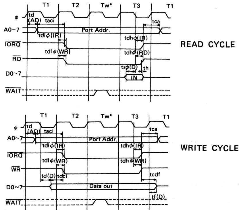
Fig. 5-3 I/O WRITE AND READ CYCLES
