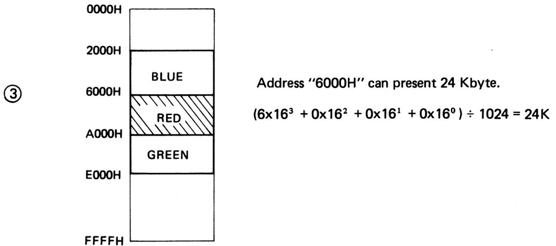
By indicating in the above memory map, address "6000H" is the forefront address of Red video RAM memory. From the result of the address analysis No. 3, it is obvious that the defective RAM IC is one of the Red video RAMs (RAM9 ~ RAM 16. Refer to the circuit diagram No. P1126).
