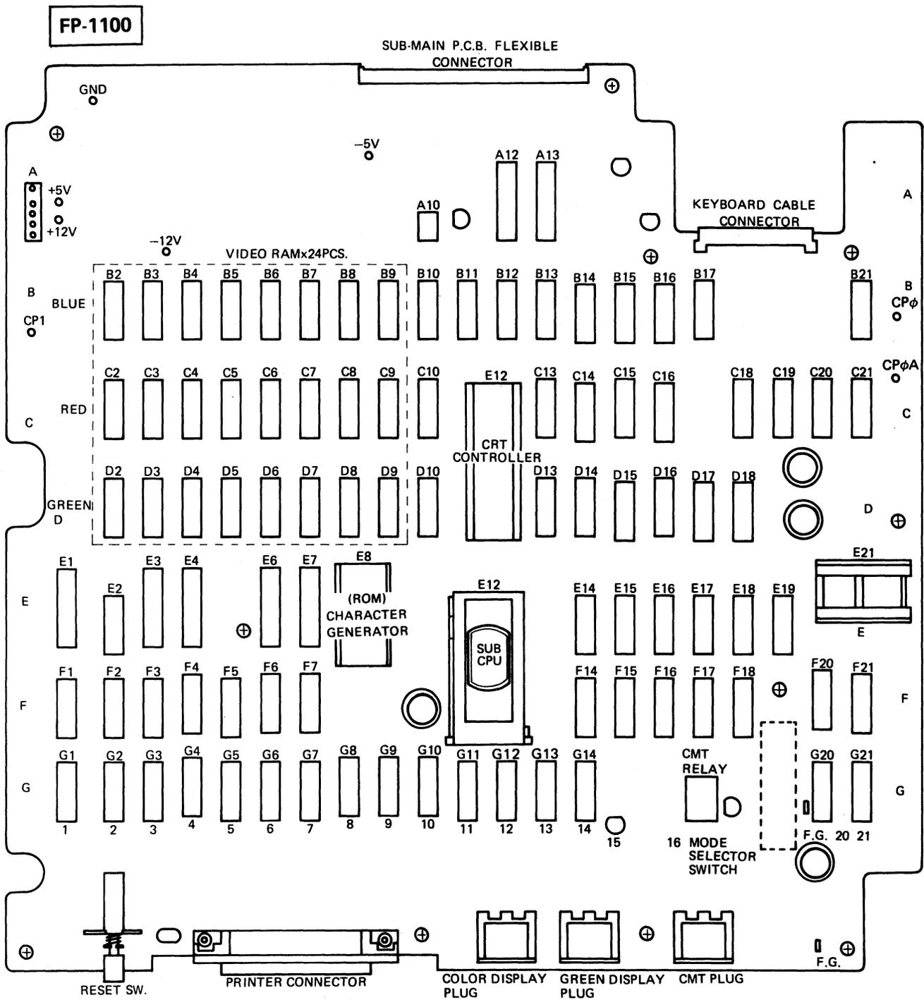
Fig. 7-2 IC LAYOUT ON THE SUB P.C.B.
