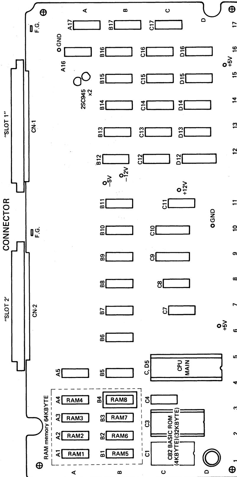
Fig. 7-1 IC LAYOUT ON THE MAIN P.C.B.
