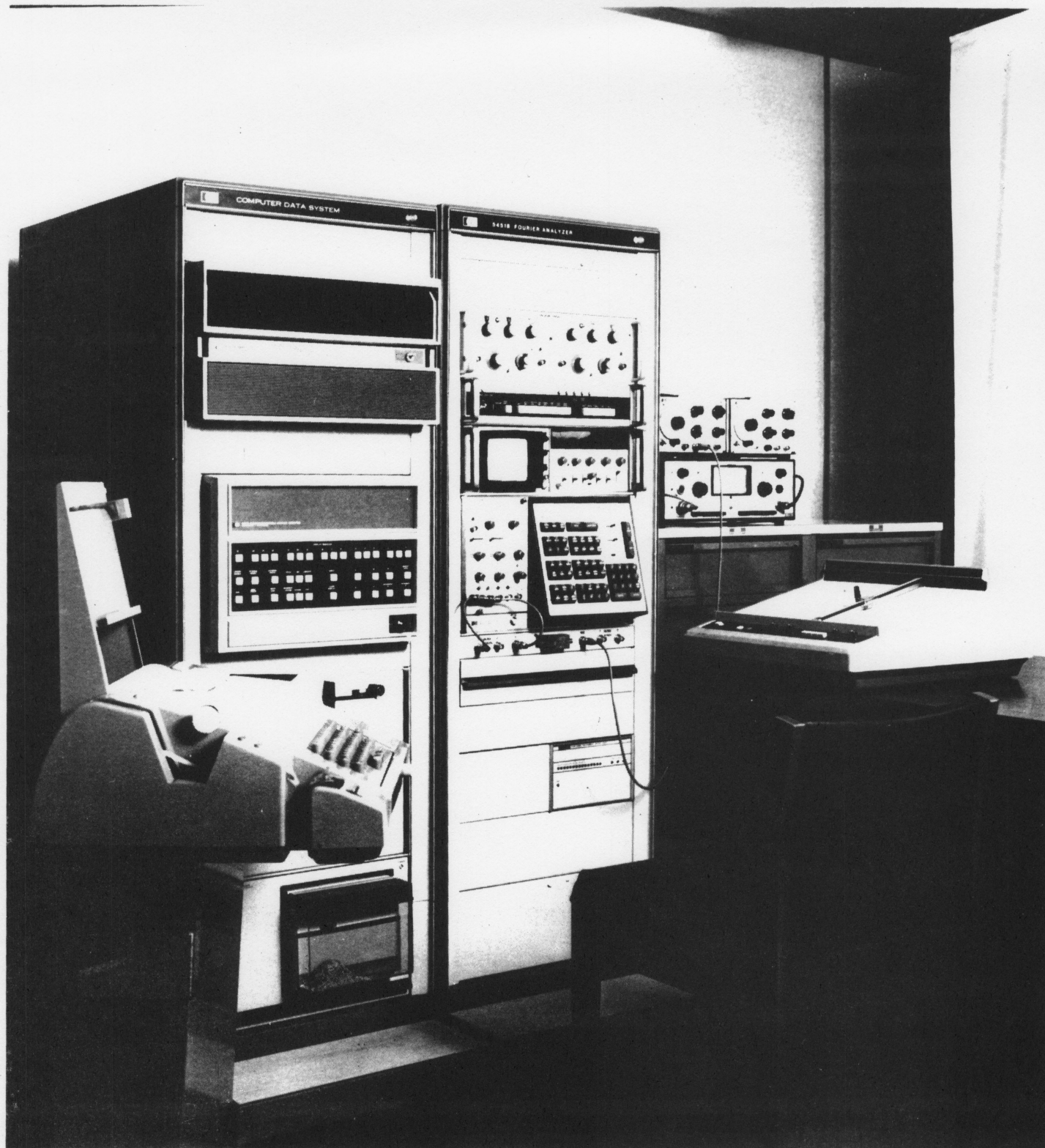
Computer equipment used by KEF for measuring impulse responses of loudspeakers and recording processed results.
