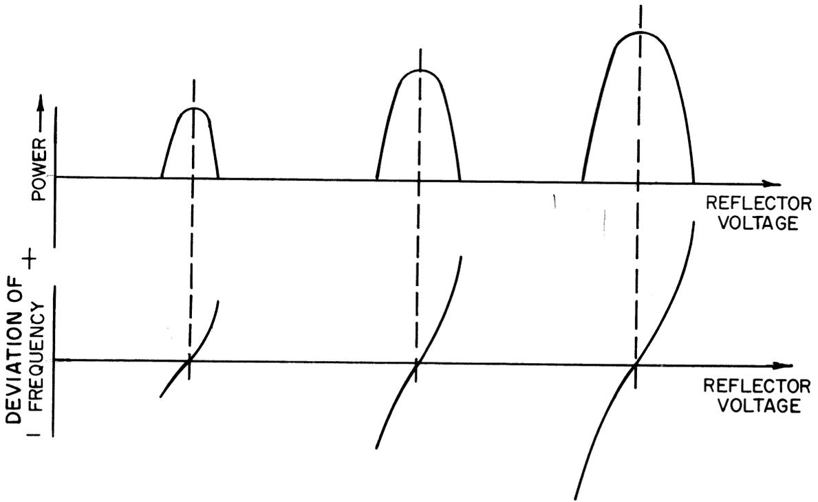
FIGURE 3: TYPICAL KLYSTRON OUTPUT, SHOWING "MODES"
