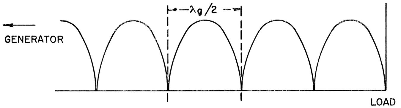
b. VOLTAGE STANDING WAVE, SHORT CIRCUIT AT LOAD END.
