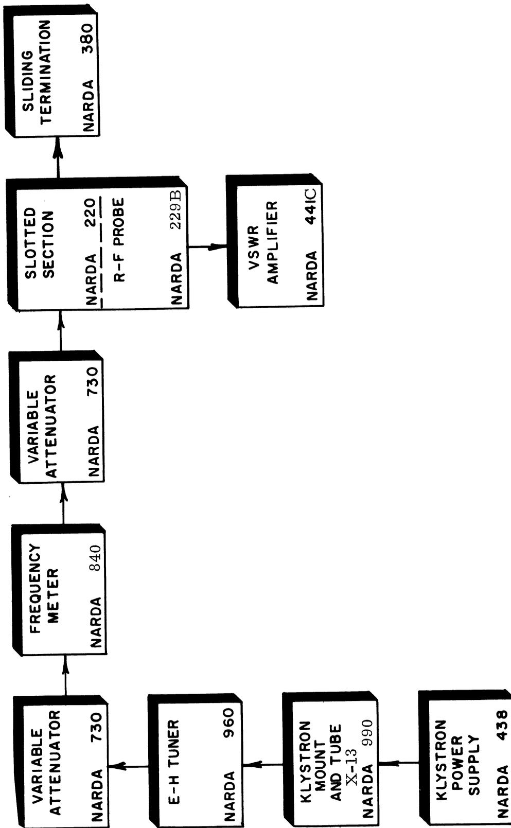
FIGURE 17: WAVELENGTH-FREQUENCY MEASUREMENTS EXPERIMENT SET-UP
