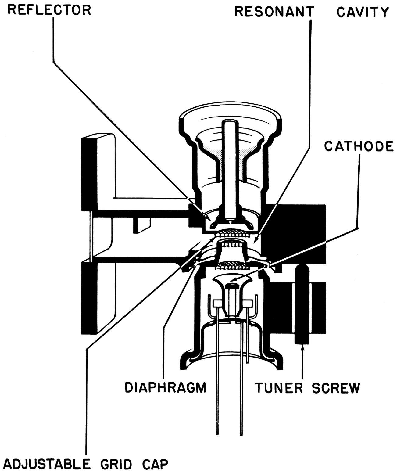
FIGURE 6B: SCHEMATIC REPRESENTATION OF KLYSTRON
