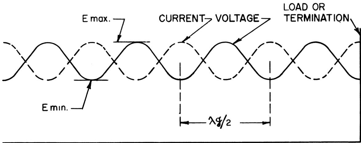
FIGURE 2: EXAMPLE OF A STANDING WAVE, VOLTAGE OR CURRENT
