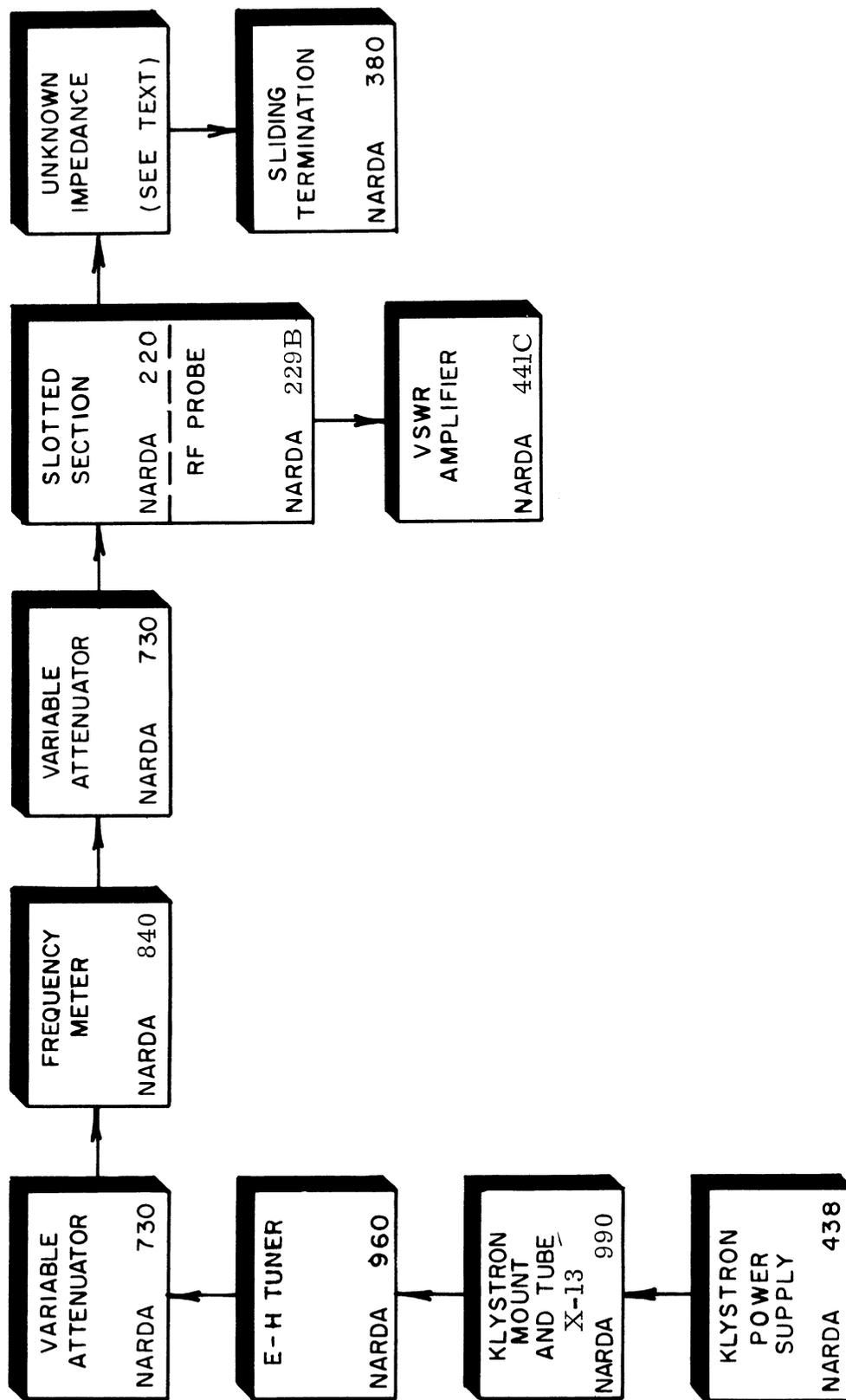
FIGURE 23: IMPEDANCE MEASUREMENT SET-UP
