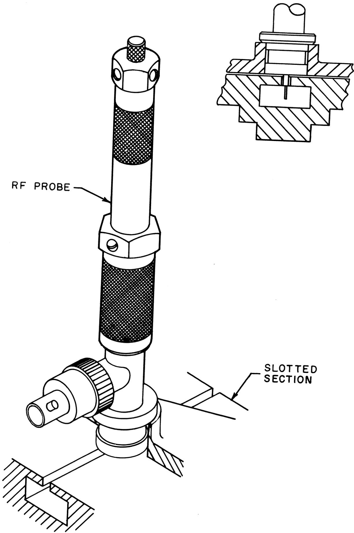
FIGURE 10: SLOTTED LINE PROBE ASSEMBLY
