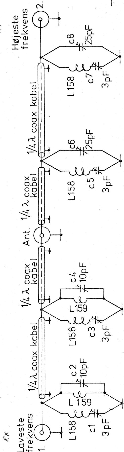
$$\text{Kabelløngde} = \frac{54}{\text{frekvens (MHz)}} \text{ m}$$
