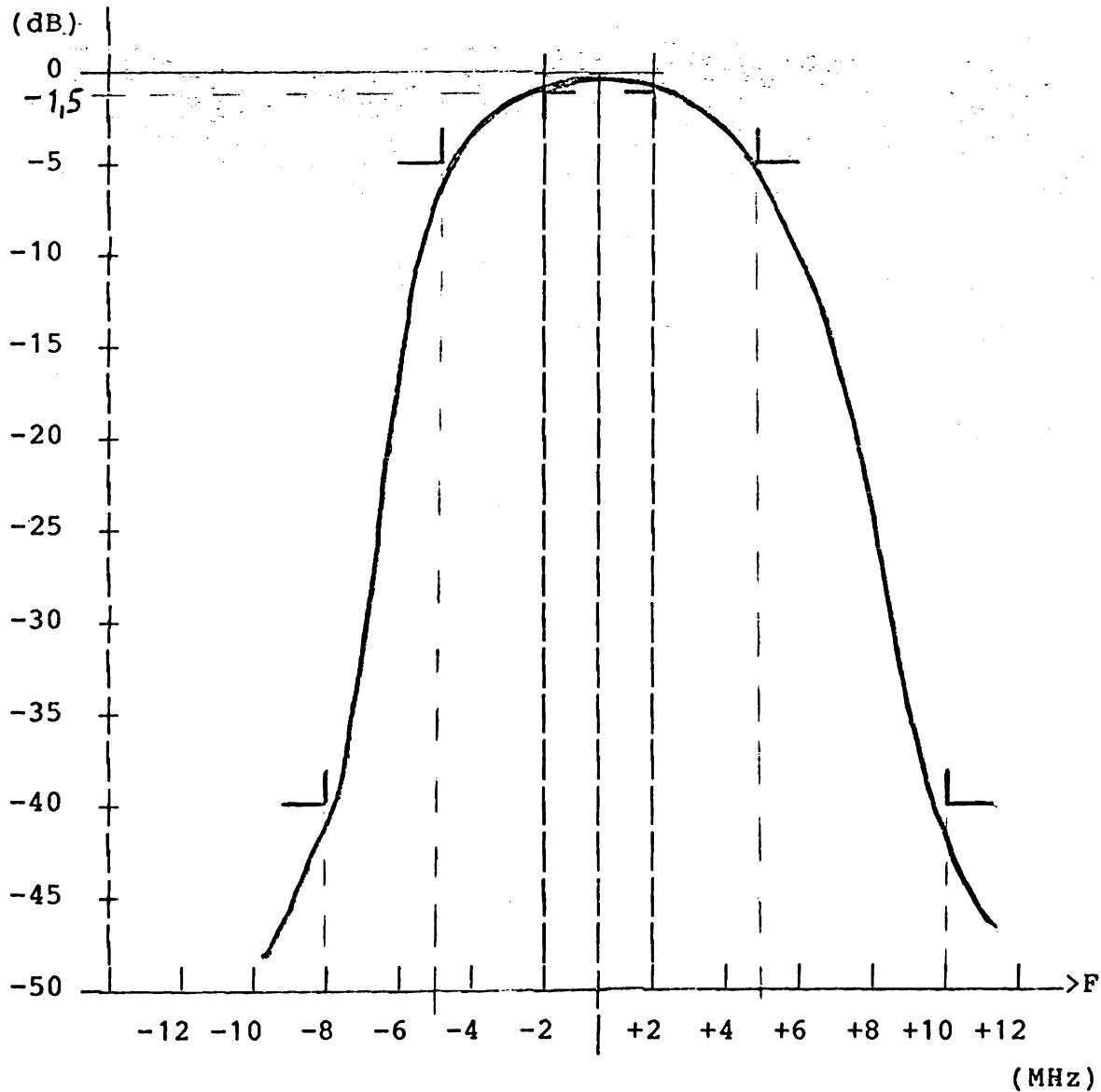
Afprøvning af Tx synthesizer for ap 3000 NMT - print N18B
