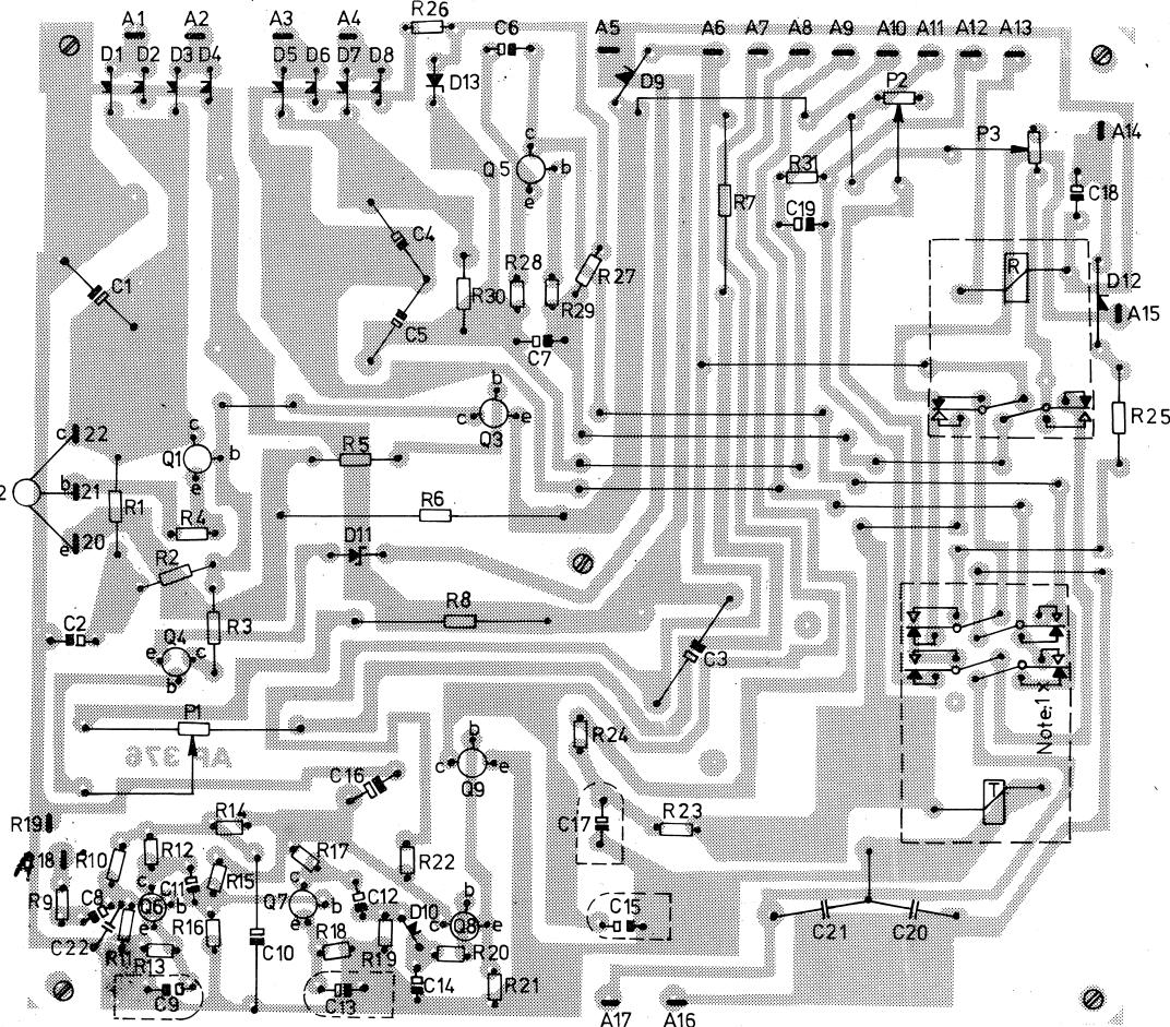
Note 1: If several RC's are to be parallel coupled disconnect print at mark "X"
