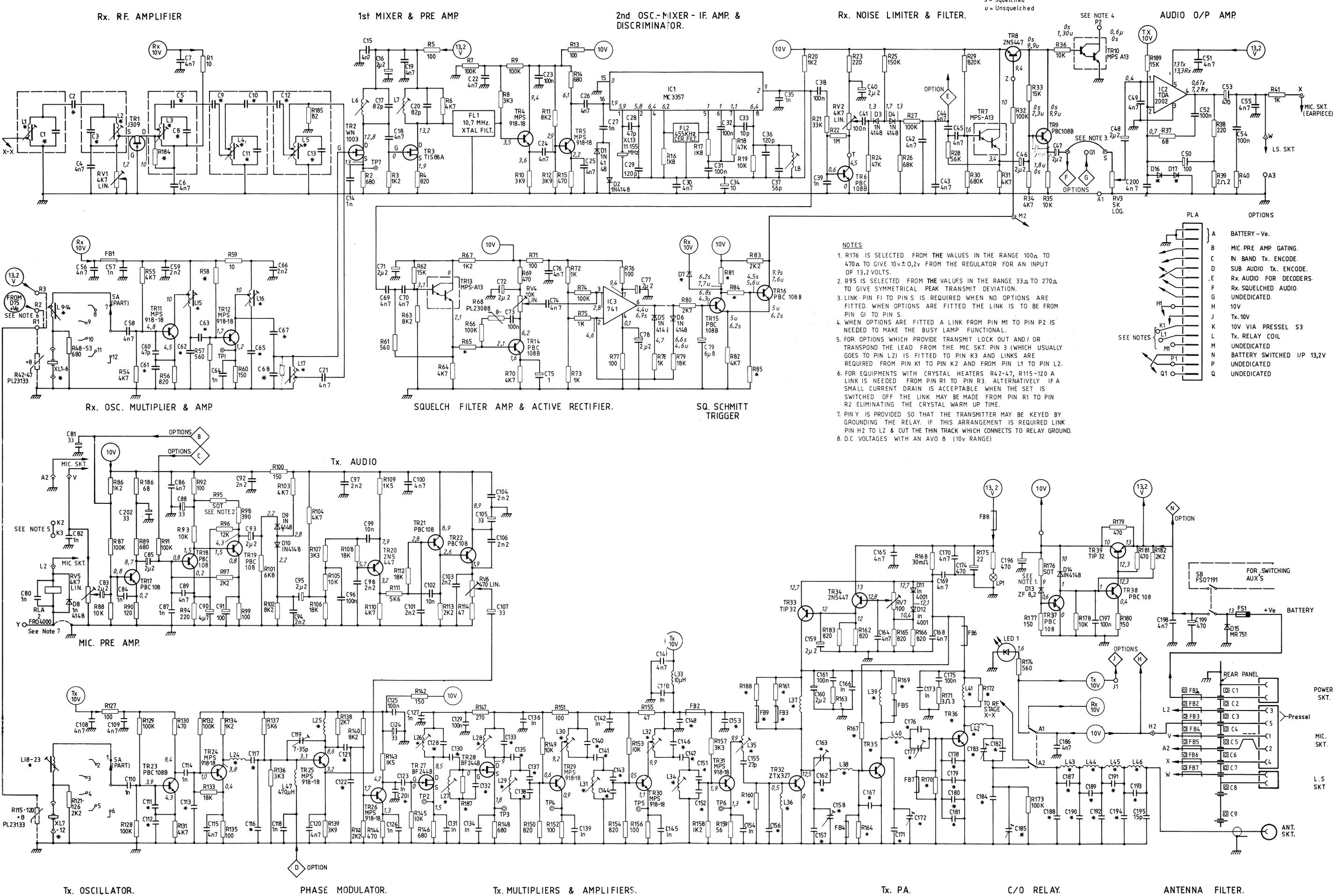
**FIG 6:3 OVERALL CIRCUIT DIAGRAM M294 TRANSMITTER/RECEIVER**
