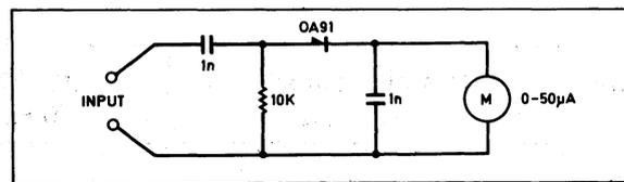
Fig. 4.1 Diode Probe Circuit Diagram
