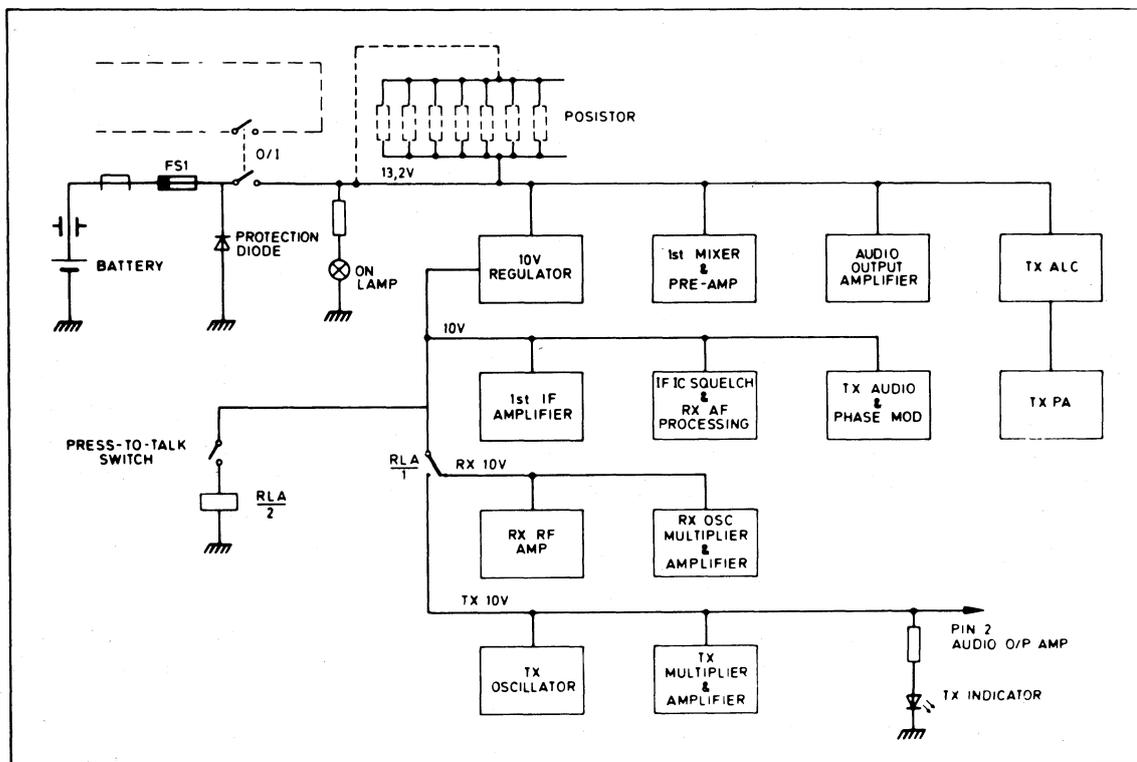
**Fig. 3.2 Power Supplies and Switching**
