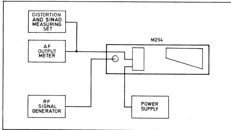
Fig. 4.2 Connection of Test Equipment – Receiver Testing
