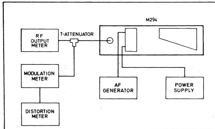
Fig. 4.3 Connection of Test Equipment – Transmitter Testing
