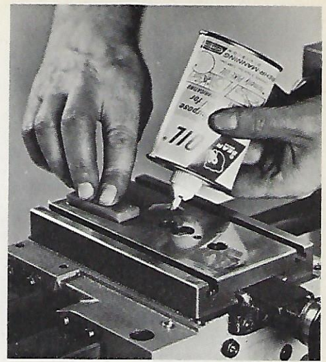
HONE NICKS on surface of carriage worktable flush with a Hard Arkansas stone.
