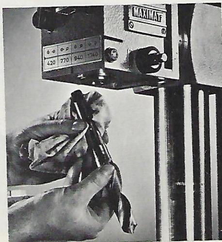
CAREFULLY CLEAN taper-shanked tools and spindle's internal taper before inserting.
