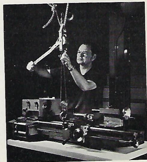
SMALL CABLE HOIST facilitates lifting lathe. Use eye bolt with cleat under bed.
