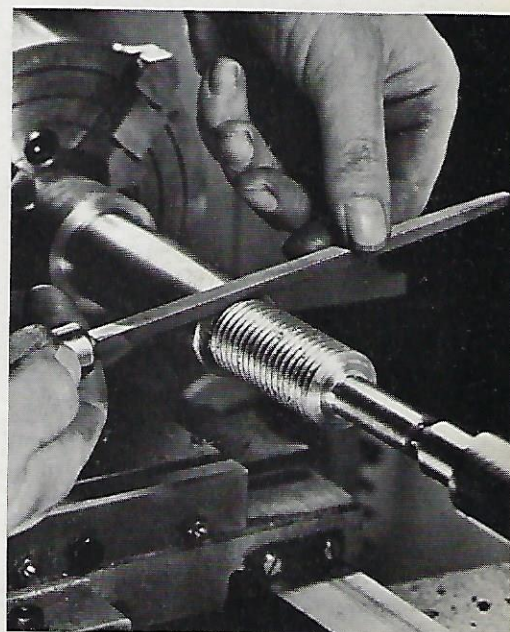
SMOOTH UP cut thread with a triangular file, rounding crests slightly. Chamfer end.
