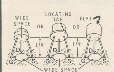
(✓) MPSA20 (#417-801) transistor at Q5 and Q6.
