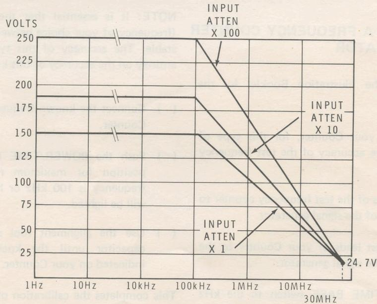
**MAXIMUM INPUT VOLTAGE DERATING CURVE**
