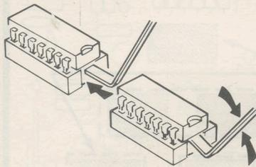
2. Refer to Detail 2-5A. Then, as you install each IC in the following steps, position the pin 1 end of the IC at the end of the socket where the dot is screened on the circuit board. Then insert the IC leads into the socket and push the IC down into place.
