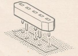
( ) D106: Mount the LED with three fiber washers. Position the flat as shown. Then solder the leads to the foil and cut off the excess lead lengths.
