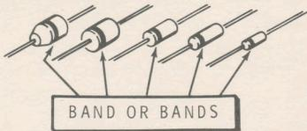
When you install diodes, always position the banded end as shown on the circuit board.
