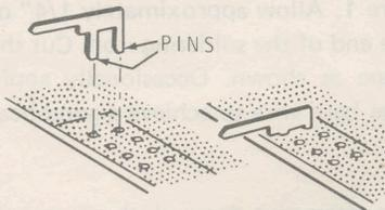
( ) Position the display circuit board as shown and install 30 F connectors.
