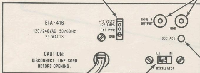
**OSCILLATOR EXT INT switch:** Selects either the internal time base or an external time base signal.
