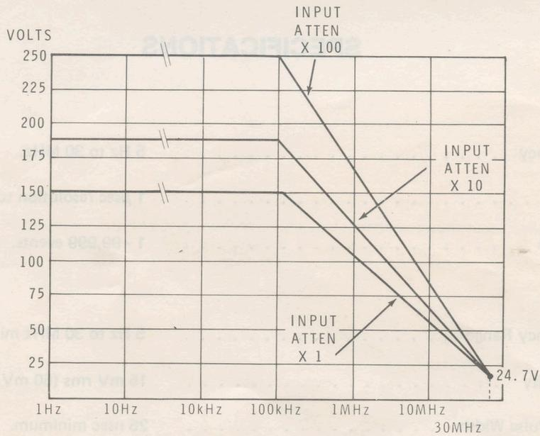
**MAXIMUM INPUT VOLTAGE DERATING CURVE**
