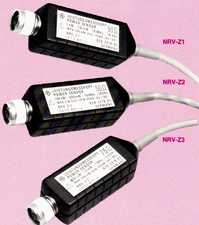
Power sensors for different impedances (50 Ω, 75 Ω) and power ranges (400 pW to 500 mW)
