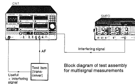
Test assembly with Signal Generator SMPD and Radiocommunication Tester CMT for multisignal measurements
