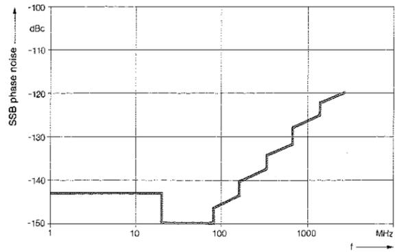
Typical values of SSB phase noise of SMPD in dBc (1 Hz) as a function of frequency; carrier offset 20 kHz
