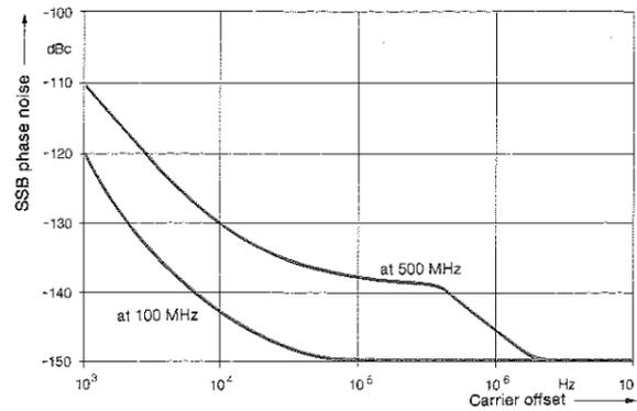
SSB phase noise of SMPD as a function of carrier offset (bandwidth 1 Hz)
