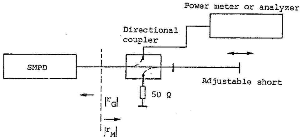
Settings on the SMPD: Test frequency 300 to 2720 MHz, unmodulated
