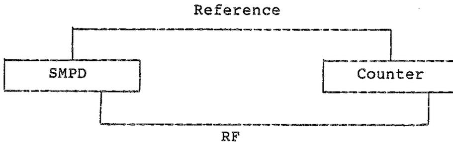
Synchronize the reference frequencies of SMPD and counter. Set level on the SMPD at which the counter operates properly. Set the frequencies to be checked. The last digit of the values read off the counter may deviate by  $\pm 1$ .
