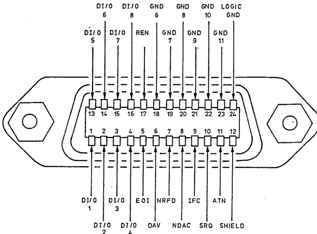
Fig. 2-3 Pin assignment
