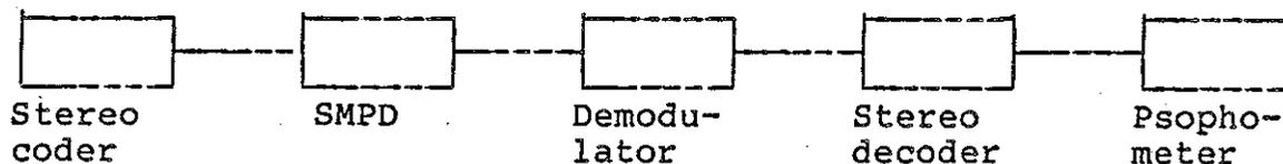
Modulate only one channel with 40 kHz deviation and a modulation frequency of 500 Hz. Select a pre- and deemphasis of 50  $\mu$ s on the stereo coder and decoder respectively. Make sure that the stereo signal is to standard. Read the reference level on the psophometer. Remove stereo coder and short-circuit FM input socket 31 on the SMPD. The unweighted S/N ratio is indicated on the psophometer. The difference between measured and reference level should be  $>76$  dB.
