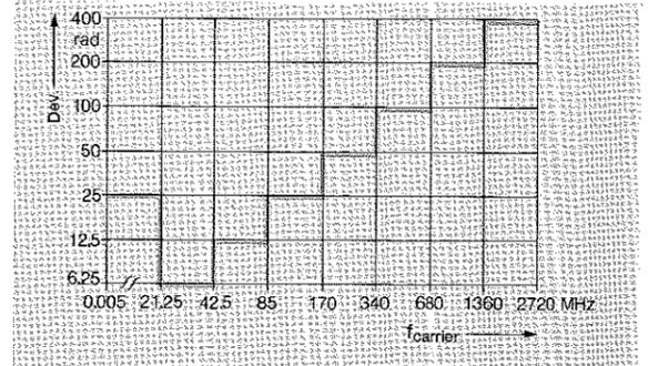
Maximum adjustable deviation as a function of carrier frequency
