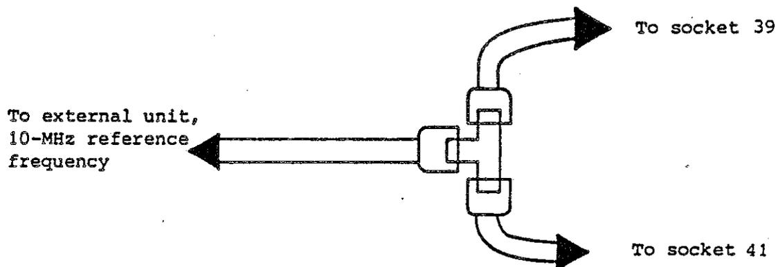
Fig. 2-2 Feeding an external unit
