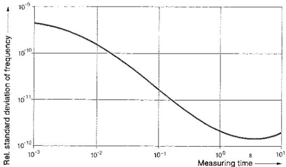
Relative standard deviation of frequency of SMPD at 1360 MHz (internal reference frequency) as a function of measuring time
