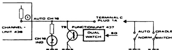
When the line AUTO CH is "open" (5 V) and the CH 16 indicator is alight, the channel switches are open, and a logic code for word 26 in the PROMs appears. See connections pin 4, 9, 13 CHANNEL-UNIT 436.
