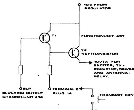
When the KEY is pressed, the POWER RELAY is activated (only on 25 W) and the KEY TRANSISTOR (when not blocked) will feed the EXCITER with 10 V.
