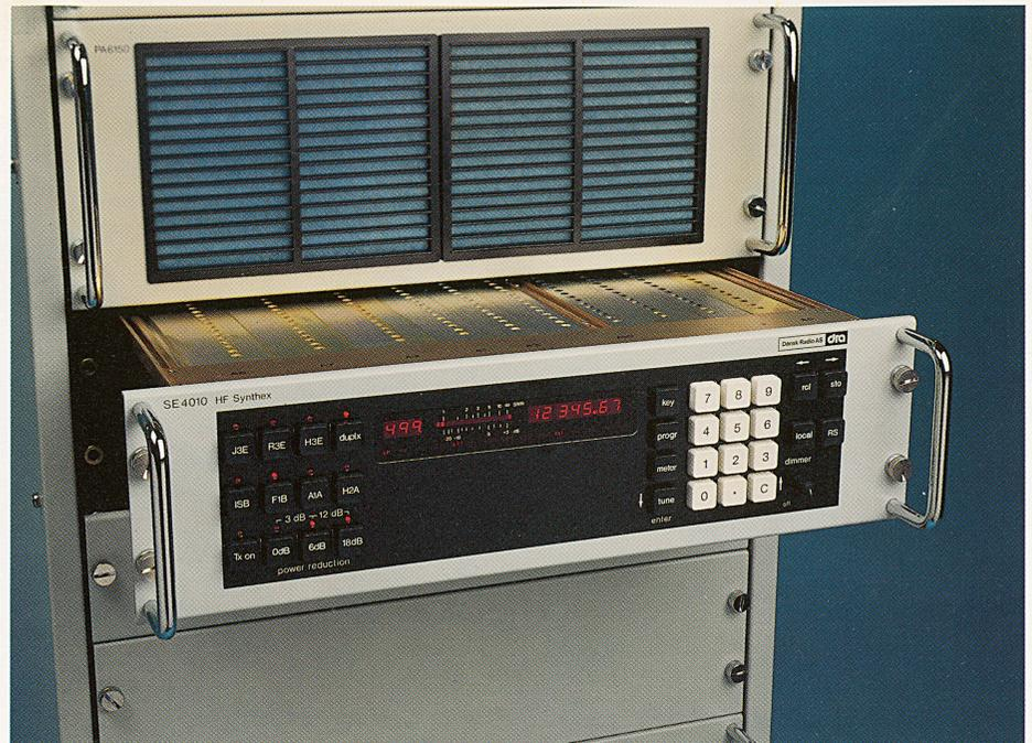
Synthesizer SE 4010 synthesized exciter. Frequency range 1.5 to 30 MHz. Ask for separate leaflet.
