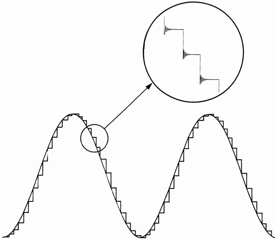
Fig. 3.3 - Typical DAC Output Waveform
