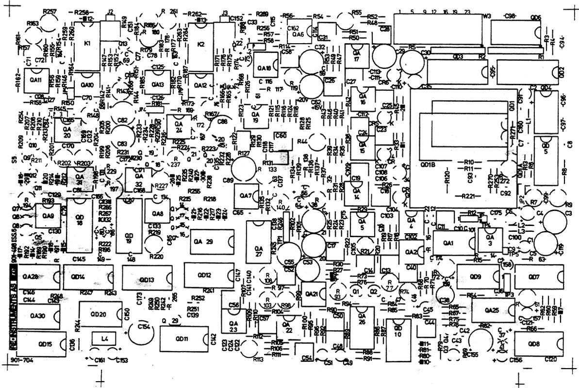
Fig. 3.5 - Analog Board Component Layout
