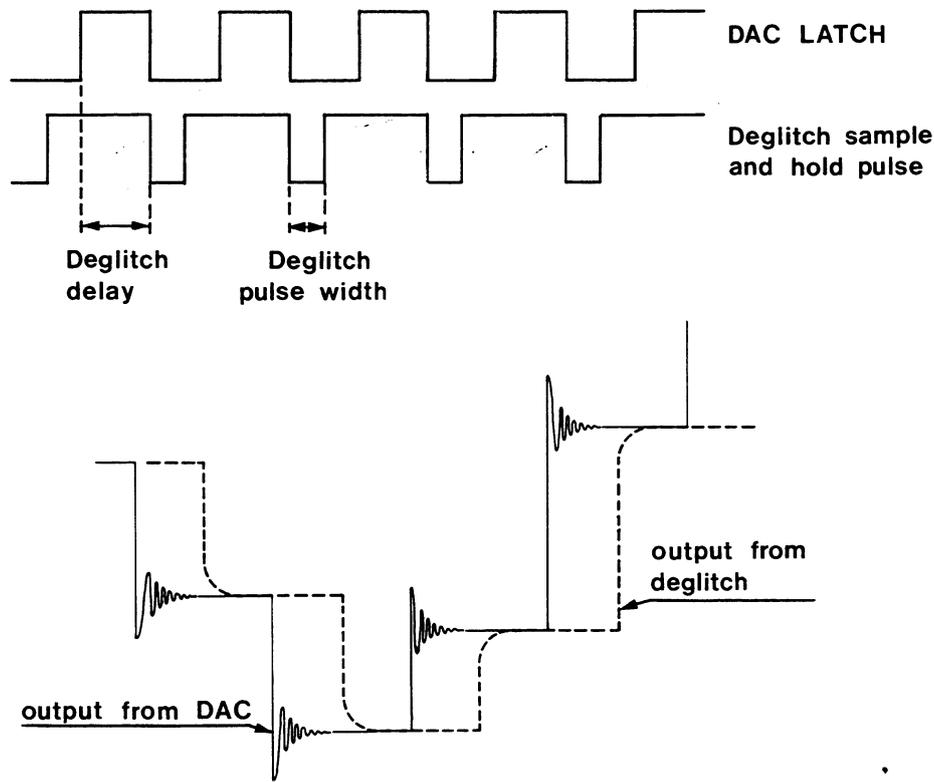
Fig. 3.4 - Function and Timing of Deglitch Network
