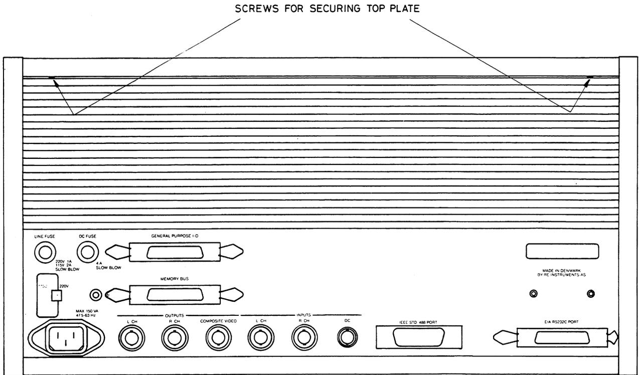
Fig. 1.1 - Top Plate Screws
