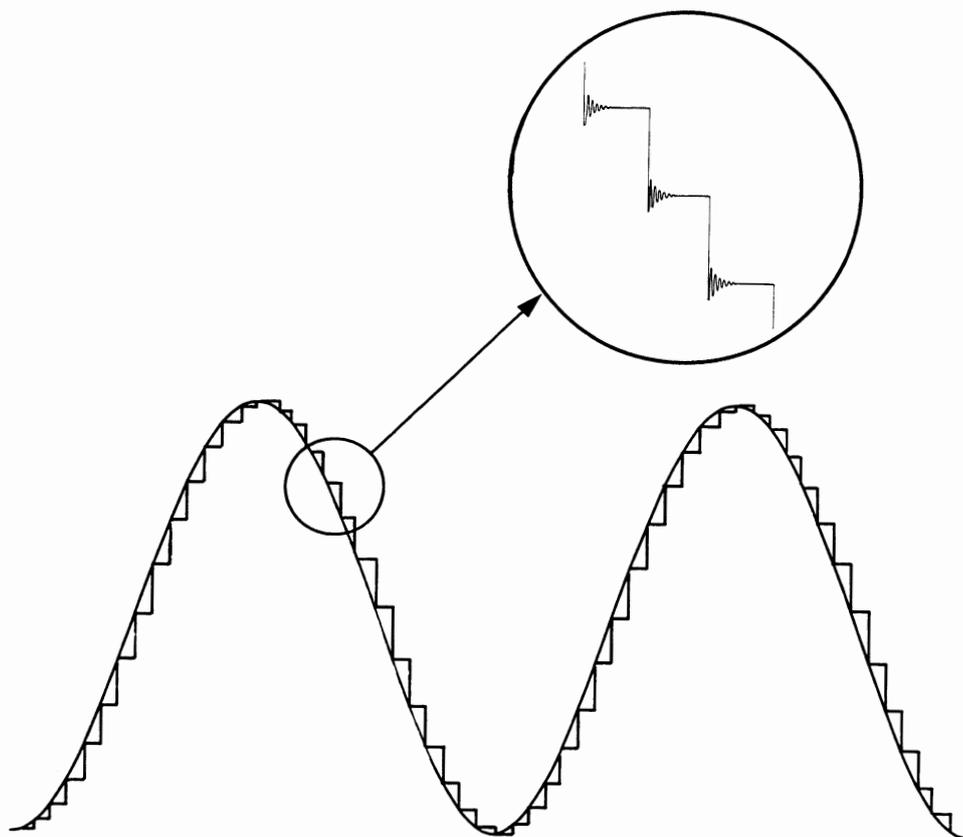
Fig. 3.3 - Typical DAC Output Waveform
