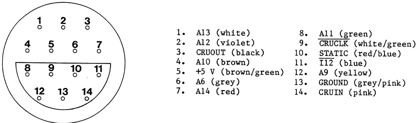
Fig. 2.1 - RE905 Keyboard Connector Pin-out
