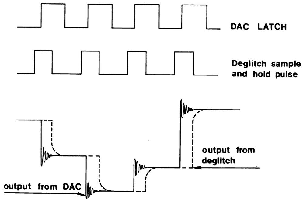
Fig. 3.4 - Function and Timing of Deglitch Network
