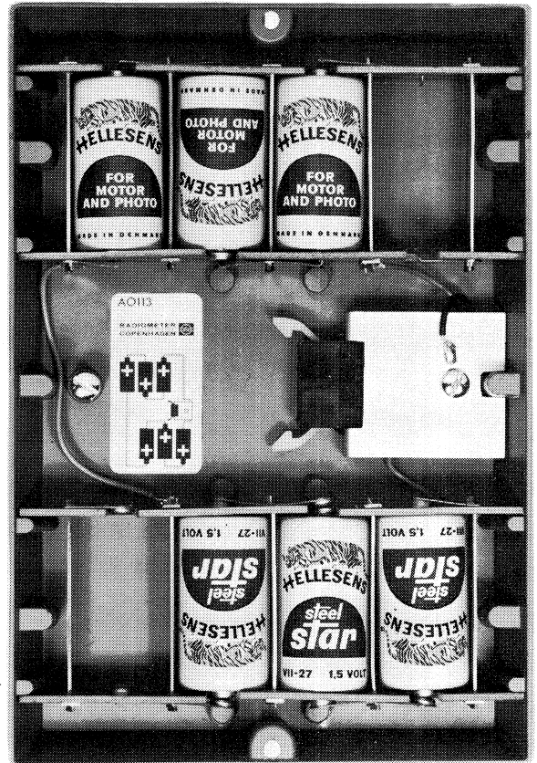
Fig.D2. Interior of Power Supply, type AO113, showing battery positions and socket of connector from Power Supply Unit to Electronic Galvanometer.
