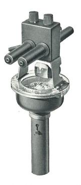
Sailor Ferrite Navigator. The Sailor ferrite direction-finder is rotatably mounted on a graduated plotting ruler. The ferrite Navigator is placed direct on the chart, and is movable on a pin placed on the chart where the given radio station is situated. The ferrite direction-finder is tuned to the radio station frequency and turned till minimum signal is indicated. Then the ruler is set at the course steered, and now the position line can be drawn on the chart.
