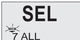
The handset display shows the message “SEL”ect and the MEM symbol flashes. The lower part of the display shows the scan table’s number and name.
