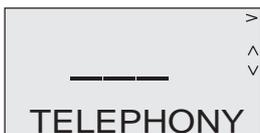
When a control unit is master of the system, the other control units, if in VHF mode, show the following display to indicate that the transceiver is in use by another control unit:
