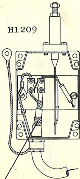
Outer screen must not be connected to ground.
