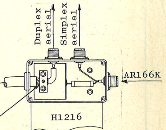
Screens must be soldered to tinplate
