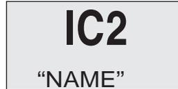
If the intercom attempt is not answered within 30 seconds, the unit automatically hangs up and reenters normal VHF operation.
