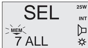
The VHF set display shows the message "SEL"ect and the MEM symbol. The lower part of the display shows the scan table's number and name.
