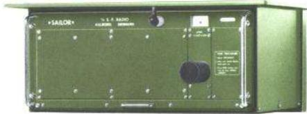
Transmitter T1127 mounted at the base point of the aerial.
