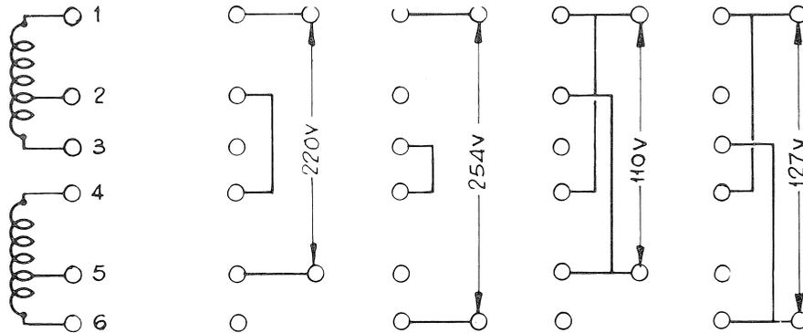
The transformer TR1402 supplies all voltages to the transmitter except filament voltage, and this transformer is connected, when either the button SIMPLEX or the button DUPLEX is pressed.
