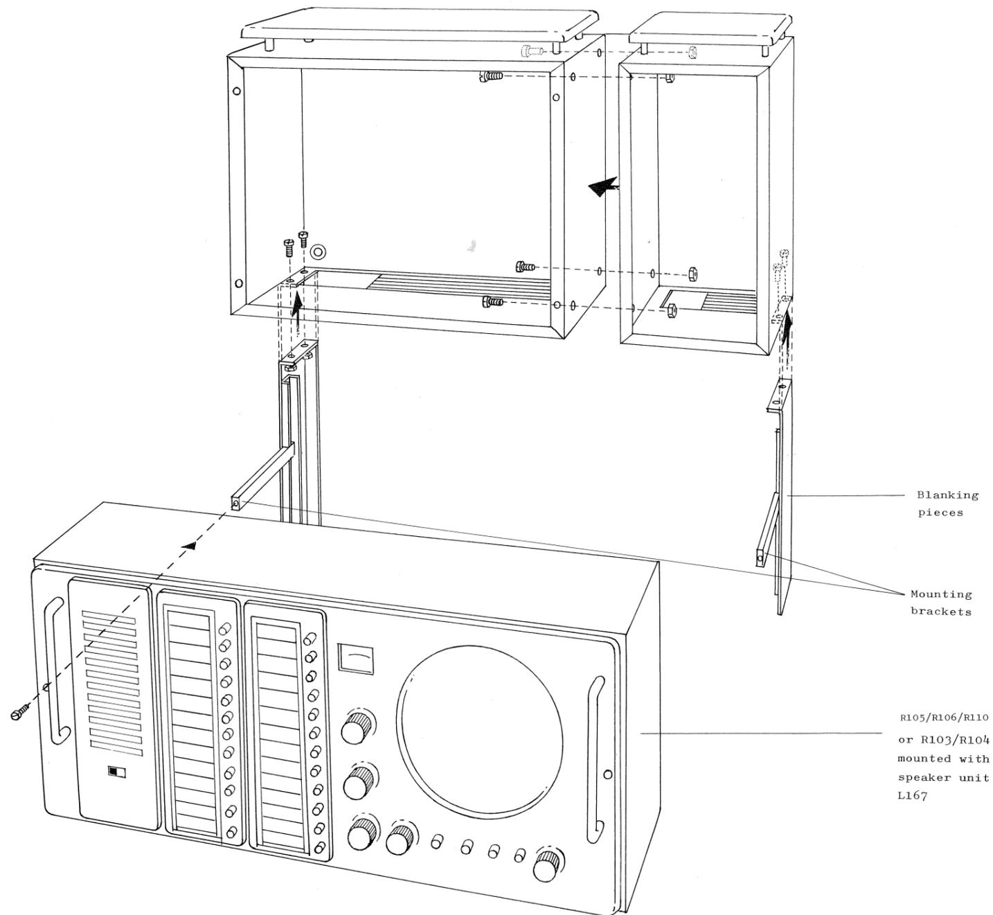
The transmitter case is fastened to the bulkhead in the normal manner utilising the four mounting holes in the back of the case. Take the power supply out of its case and mount the case on the side of the transmitter case using the four screws provided.
