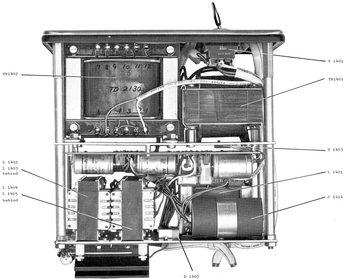
Figure 7 220/110 VAC Power supply
