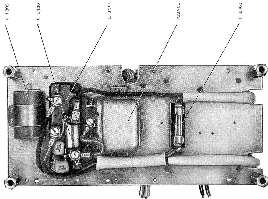
Figure 9 24VDC Power supply
