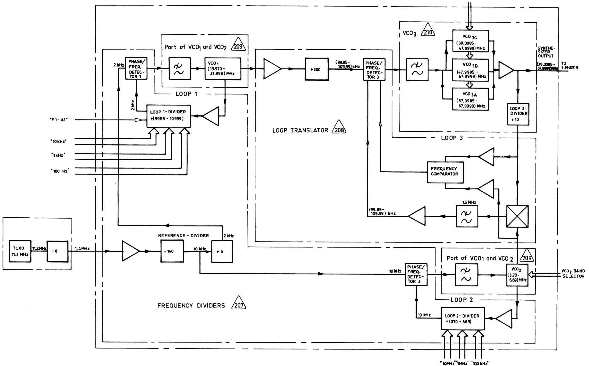
BLOCK DIAGRAM, FREQUENCY SYNTHESIZER
