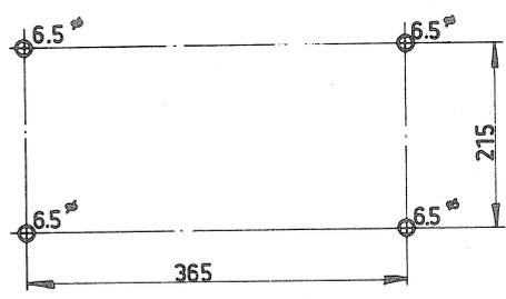
Horizontal drilling plan for bench mounting
