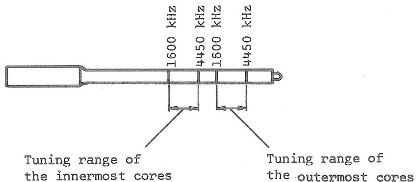
The marks on the trimming tool refer to the front of the channel oscillator printed circuit board and the edge of the coil former respectively.
