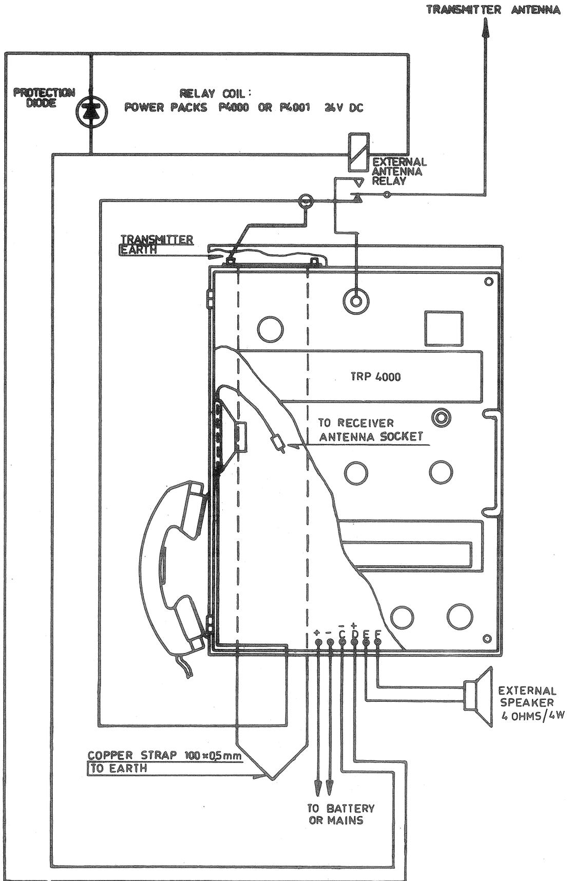
Installation of external antenna relay for extra receiver or integral receiver (simplex one antenna installation)
