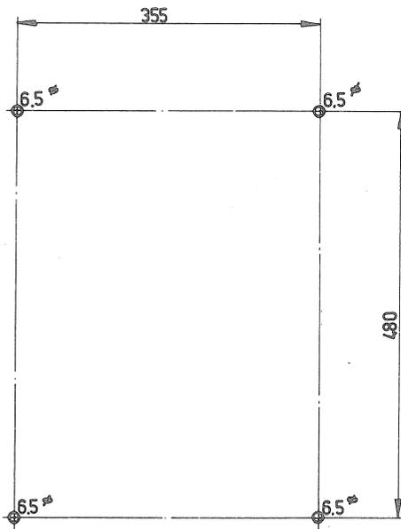
Vertical drilling plan for bulkhead mounting
