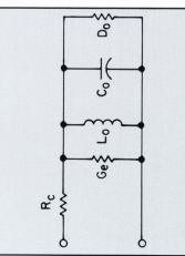
Figure 1. Equivalent circuit of an air-core inductor.  $R_{\rm c}$  is the series resistance.  $G_{\rm s}$  is the conductance due to eddy-current loss, and  $D_{\rm o}$  is the dissipation factor of the distributed capacitance.
