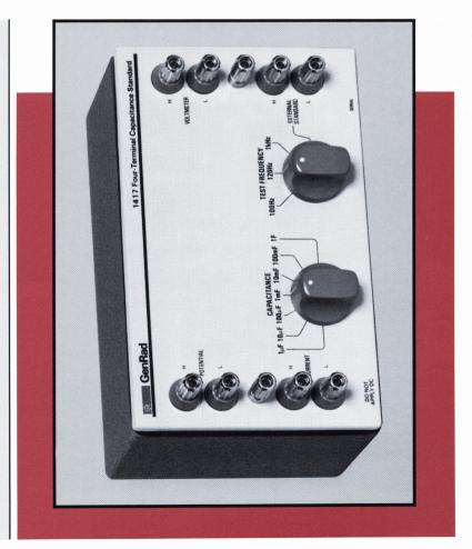
The GenRad 1417 Four-Terminal Capacitance Standard consists of a 1  $\mu$ F standard capacitor and two precise inductive voltage dividers, which scale the value of the capacitor tor up to 1 F in decade steps.
