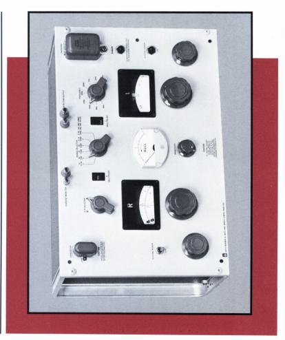
The GenRad 1633-A Incremental-Inductance Bridge is designed for measuring inductance and loss of transformers, chokes, and similar components at very high levels of ac and dc excitation. It functions over a wide frequency range from 20 Hz to 20 kHz. Other nonlinear elements such as rectifiers and lamps can also be measured.
