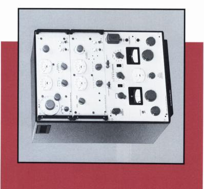
Designed to measure the inductance and loss of coils with ferromagnetic Audio Oscillator/Power Amplifier in able DC Power Supply, and 1308-A a self-contained cabinet-type rack Inductance Bridge, 1265-A Adjustthat includes all necessary cables. Inductance-Measuring Assembly consists of a 1633-A Incrementalcores, the GenRad 1630-AV
