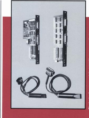
Clockwise from upper left: 1.0 V Measurement Probe, 1689-9620 High-Speed Interface, 1658-9620 Interface, and the 0.01 V Measurement Probe.
