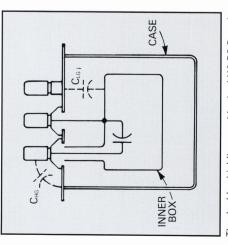
The double shielding used in the 1412-BC Decade Capacitorees Gie very small. This capacitance is the difference between the 3-terminal and 2-terminal capacitance of the box;  $C_{LG}$  is approval 56 pF.
