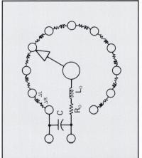
Equivalent circuit of a resistance decade, showing residual impedances.
